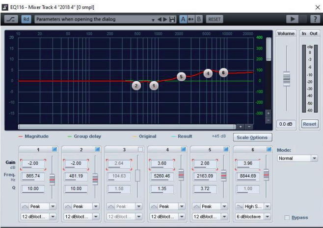
Figure 12. Equalizer for additional fine enhancement of the high end
